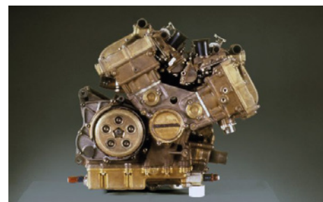
The first Honda V4 engine developed in 1978 for the Road Racing World Championship
